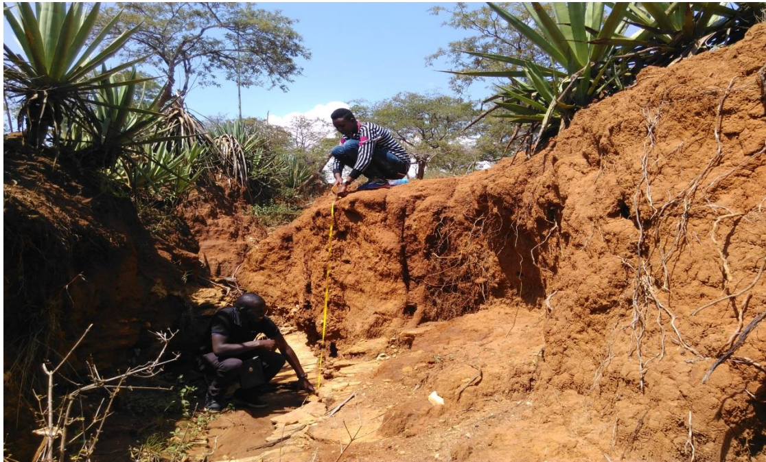
Picture 1: Measuring the Depth of Gully in Cherubei Village, Mt. Elgon Ecosystem
